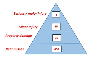
This diagram is Bird's Triangle (1969). It was devised as a result of extensive research into accidents and accident ratios. It has been determined that for every one serious injury, there will have been 10 minor injuries, 30 property damages and 600 near misses.
